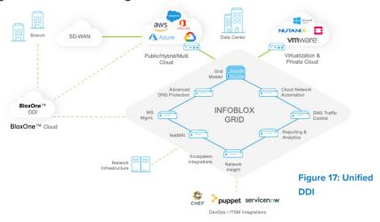
To strike the fine balance between cloud-managed DDI and local survivability, unified DDI can be configured using lightweight commodity appliances sited on location. This helps ISVs and enterprises to build upon the existing on-premises DDI components and leverage cloud computing features. A strong selling point of unified DDI is that customers can continue using their current on-premises DDI solution as they migrate to cloud-managed DDI. In this way, organizations can:
