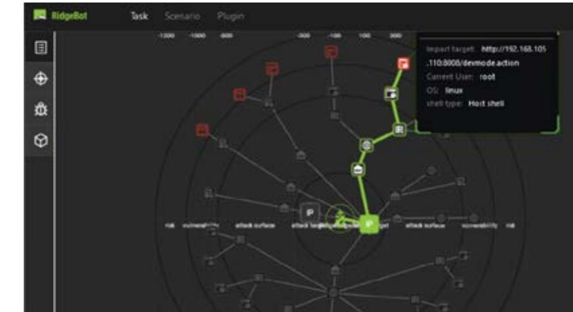
Drilling down on the exploit-path (green boxes) to the compromised target machine (red box), discloses the attack path the threat actor exploited to reach the target.
