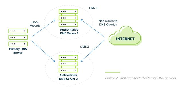
This architecture isolates the primary source of DNS records from potentially dangerous Internet traffic. Using multiple authoritative DNS servers, each with its own Internet link, creates redundancy that prevents the failure of one server or one connection from interrupting access to services.
