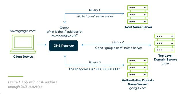
The resolver repeatedly obtains destination IP addresses and updates its cache. It is called a "recursive DNS server" because it uses recursion to perform the resolution process. Once the resolver obtains the IP address requested by the client device, that client can begin communicating with the intended domain.
