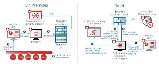
Figure 1. Solution reference architecture depicting the integration between Infoblox DDI, ActiveTrust and ActiveTrust Cloud, and McAfee security solutions.
